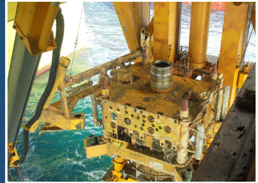
Photograph provided by CNOOC, showing recovery of an out of use subsea Xmas tree
