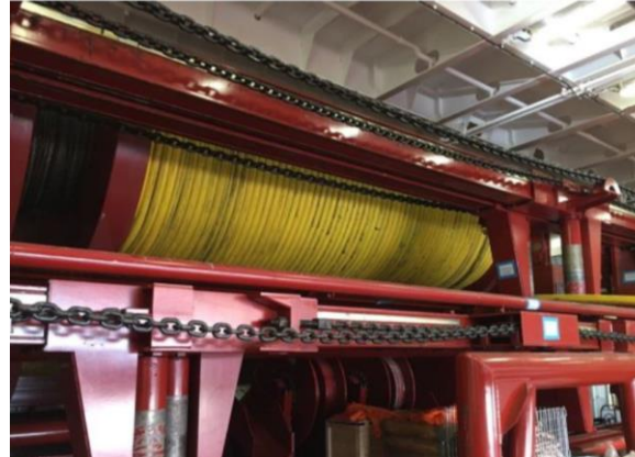
Photograph provided by Total showing Leadon flowline packed onto anchor winch drum.
